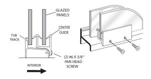
11 Slide the stainless steel bumper inserts [U] into the four soft vinyl jamb bumpers [V]. Align the slots in the bumpers with the glass panels and snap the bumpers downward over the top and bottom wall jamb screws [D] with the spacers [E].
