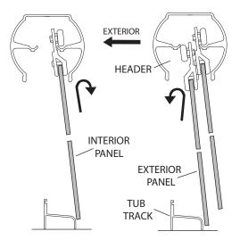
**10** Locate the nylon bottom guide [S] in the middle of the tub track [A] with the glass panels in the position shown. With a 7/64" bit, drill two holes into the V-groove through the mounting holes in the guide. Install the bottom guide with two #6 x 3/8" pan head screws [T] thru the drilled holes as shown.
