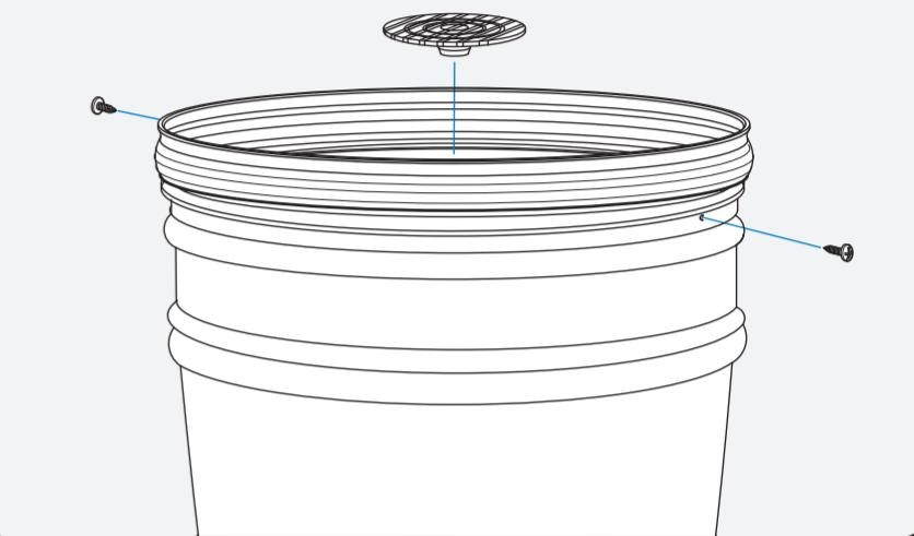
Screw here to secure lid in normal position
