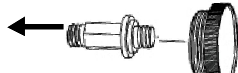
Figure 8 - Removing Regulator Cap from Pressure Selecting Screw
