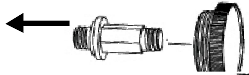
Figure 4 - Removing Regulator Cap from Pressure Selecting Screw
