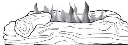
Figure 23 - Correct Burner Flame Pattern
