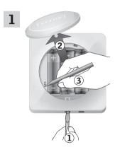
Remove the battery lid by pressing the button with a screw driver as shown in the illustration ①. ②.
