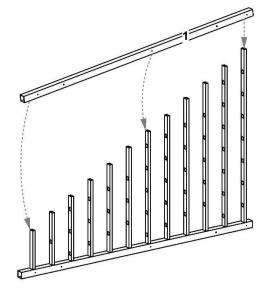
Slide left post (part 1) over corresponding support and cross rails.
