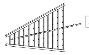
Starting with center hole, insert 84" vertical rail (part 15) through cross rails.
