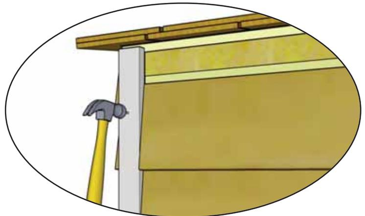
**28.** Locate 2 **Front Filler Trims (4A)** (1 1/2" x 5/8" x 65"). Filler trim will be covered by corner trim in **Step 37**. Attach in each front corner with **6 - 1 1/2" Finishing Nails (K)**.
