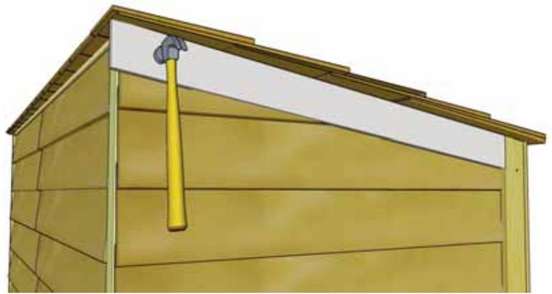
**39.** Continuing around the shed, place a **Side Facia Trim (4I)** angle cut both ends ( $1/2'' \times 2 1/2'' \times 33 7/8''$ ) tight against front side corner trim and snug underneath roof panel. Attach side facia into side wall cleats with **4 - 1 1/2'' Finishing Nails (K)**.
