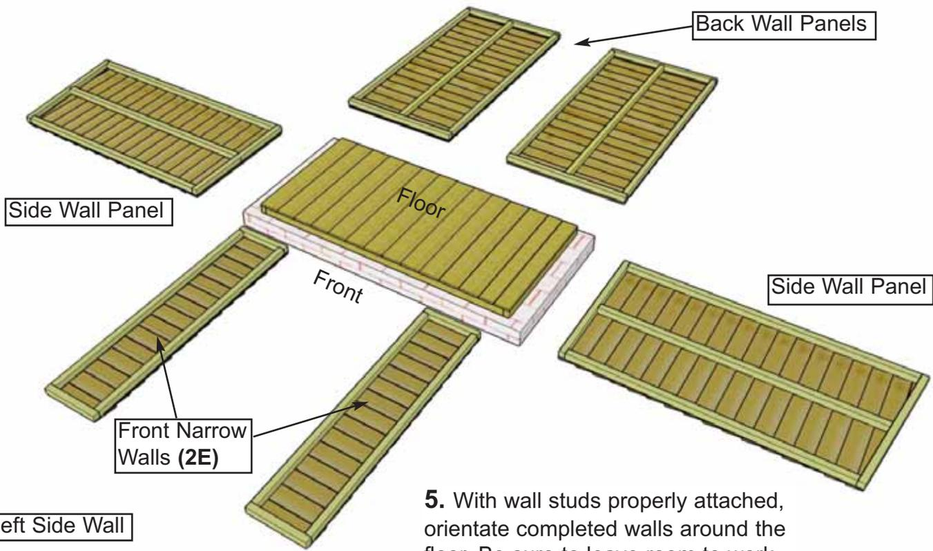
5. With wall studs properly attached, orientate completed walls around the floor. Be sure to leave room to work. **Front Narrow Wall (2E)** will be required in this section.
