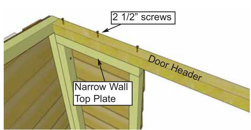
**15.** With door header positioned evenly on narrow wall top plates and flush against side wall top framing, secure using **6 - 2 1/2" Screws (C)** screwing down from the top of door header down into the upper narrow wall plates. Have your helper push side walls against end of door header to achieve tight fit if possible.
