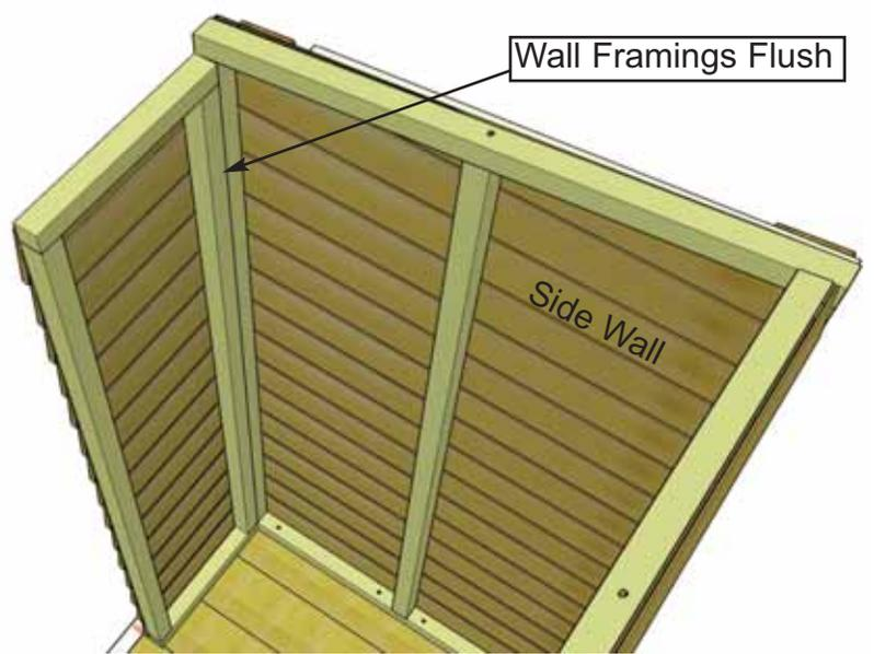
**11.** Locate **Front Narrow Walls (2E)** and position wall framing flush with side wall framing in corner. Make sure narrow wall is positioned right side up.
