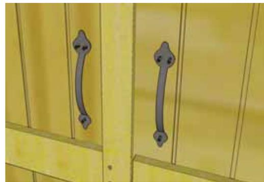
**46.** Attach **Door Handles (X)** to doors with **3 - 3/4" Black Headed Screws (J)** per handle. Choose desired handle height. Make sure screws go into interior door framing and are not exposed on inside.
