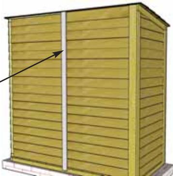
**41.** Locate **Rear Center Trim (4M)** ( $1/2'' \times 2 1/2'' \times 72''$ ). Align tight against upper rear trim and underneath roof. Attach with **6 - 1 1/2'' Finishing Nails (K)**.
