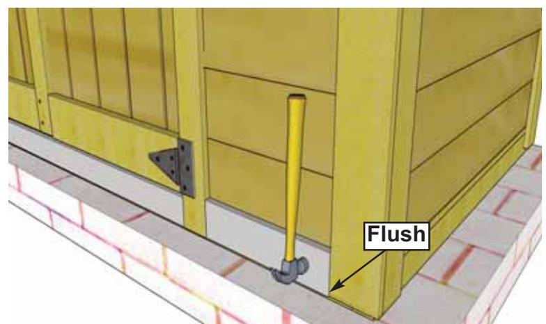
**44.** Locate both **Lower Front Narrow Trims (40)** (1/2" x 2 1/2" x 11 1/8") and **Doorway Narrow Trim (4P)** (1/2" x 2" x 40 7/8"). Place narrow wall trims between door trim and front corner trim flush with bottom of trims. Attach each with **2 - 1 1/2" Finishing Nails**. Place lower door trim between door trims flush with bottom. Attach with **4 - 1 1/2" Finishing Nails (K)**.
