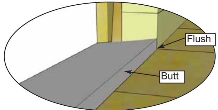
**32.** Locate **Door Threshold (4Q)** ( $1/2''$  thick at butt x  $2 5/8''$  wide x  $40 7/8''$ ). Position threshold on floor in the opening. Align with thick side of the bevel to the inside flush with the wall stud. Attach with 4 -  $1 1/4''$  **Screws (E)**.
