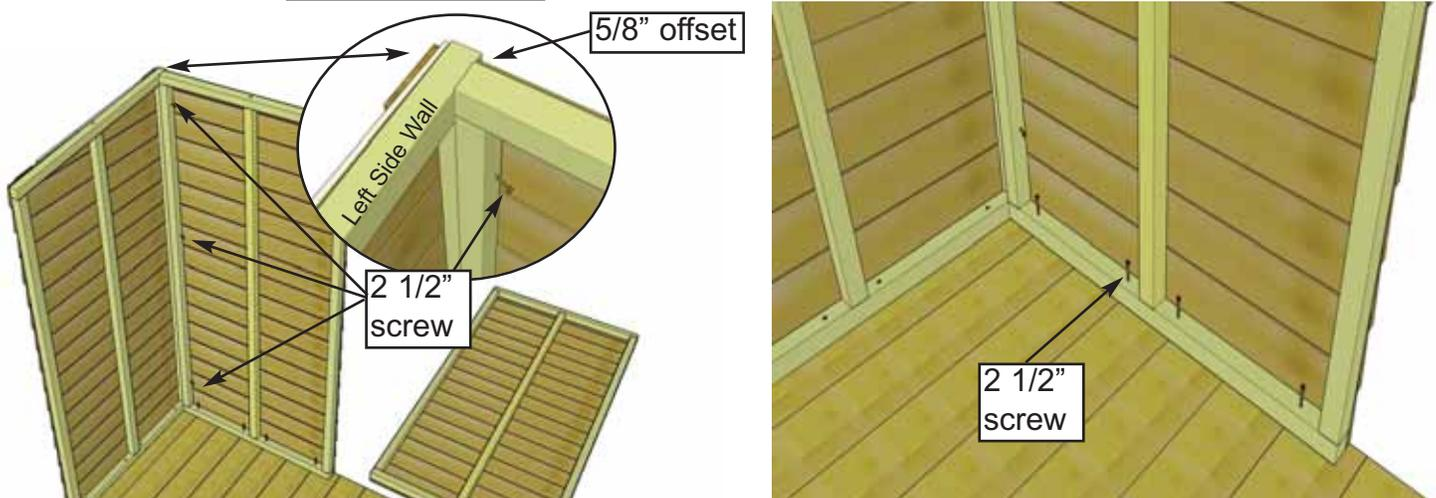
8. When side and back walls are aligned in corner correctly, wall framings will be offset. Screw wall framings together with **3 - 2 1/2" Screws (C)**. Secure bottom wall plate to floor with **4 - 2 1/2" screws (C)**.
