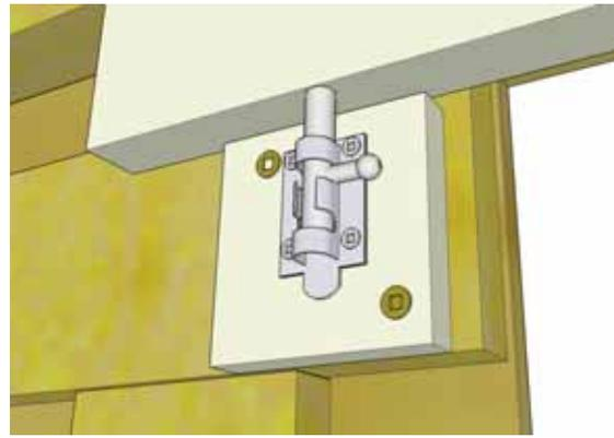
**50.** Open door and drill out marked barrel bolt impression with a 3/8" Drill Bit. Close door, slide barrel bolt in drilled hole to confirm fit.
