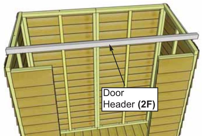
**13.** Align and attach the second front narrow wall panel as per **Step 12**.
