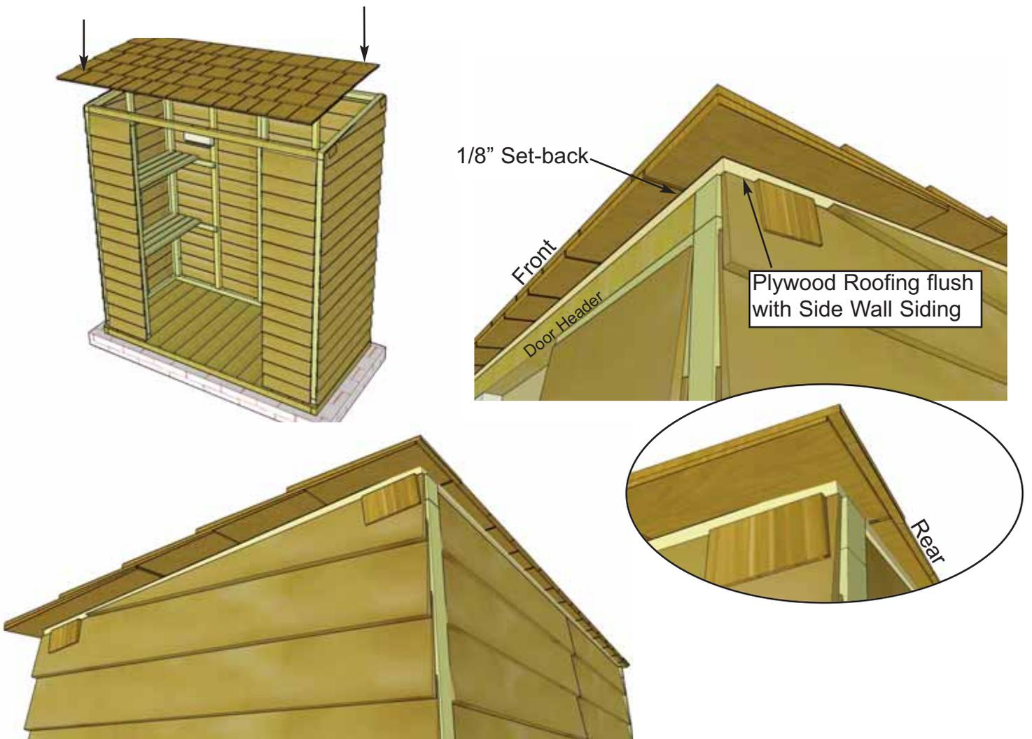
**26.** Lift up completed cedar shingle roof panel and place on upper wall framing. In the front, align plywood roofing 1/8" back from door header. On the side, plywood should be flush with side wall siding. Equally space roof from side-to-side. In the rear, plywood should sit on back wall top plate.
