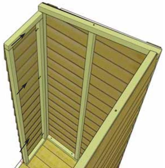
**12.** Align butt or bottom of wall siding flush with outside of floor framing. When correctly positioned, secure bottom wall plate to floor with **2 - 2 1/2" Screws (C)**. Attach vertical wall framings together at top, middle and bottom with **3 - 2 1/2" Screws (C)**.
