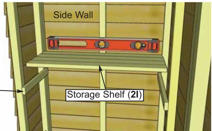
**18.** Storage Shelf positioning is flexible so decide what height configuration suits your needs. Gather your **Storage Shelf Supports (2H)**. The short Support (14 1/2") attaches to the narrow wall, the long (18 1/4") to the back wall. Position using a Level, and drill Pilot Holes to prevent ends of Supports from splitting. Attach first Support using **2 - 1 1/4" Screws (E)**. Place Storage Shelf on attached Support, Level, and mark position of 2nd Support. Pilot Hole and secure 2nd Support.
