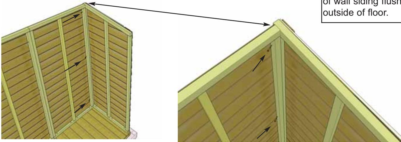
**10.** In the corner, align and attach right **Side Wall (2A)** framing to back wall framing as per **Steps 7 & 8**. Secure bottom wall plate of side wall to floor with 4 - 2 1/2" **Screws (C)**.
