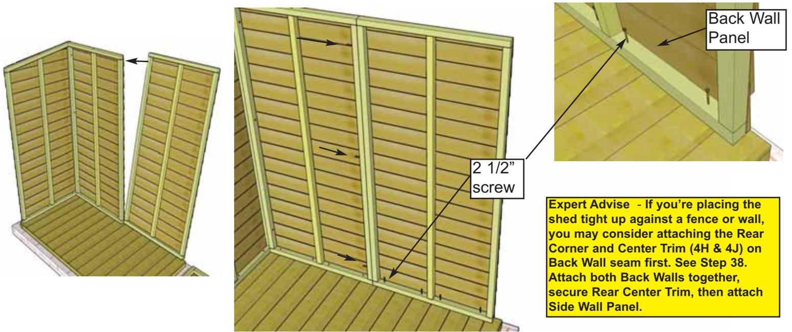
**Expert Advice** - If you're placing the shed tight up against a fence or wall, you may consider attaching the Rear Corner and Center Trim (4H & 4J) on Back Wall seam first. See Step 38. Attach both Back Walls together, secure Rear Center Trim, then attach Side Wall Panel.
