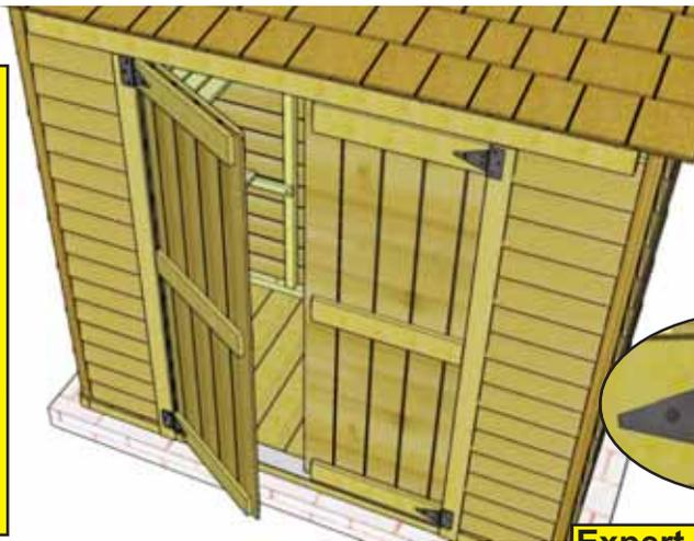
**37.** With both Doors partially attached, check to see doors open and close correctly. Make any necessary adjustments and when satisfied, completely secure hinges to vertical door frame trim with **two more 2" Black Headed Screws (H)** per hinge. Drill pilot holes to prevent wood from splitting.
