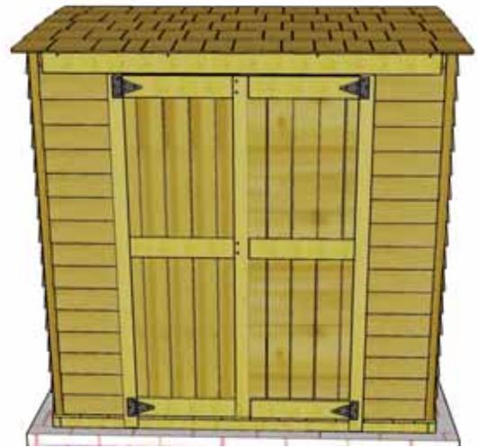
**36.** Position left side door (with flange) as per **Step 35**. Once again, use only **1 - 2" Black Headed Screw (H)** per hinge initially to secure door to vertical door frame trim.
