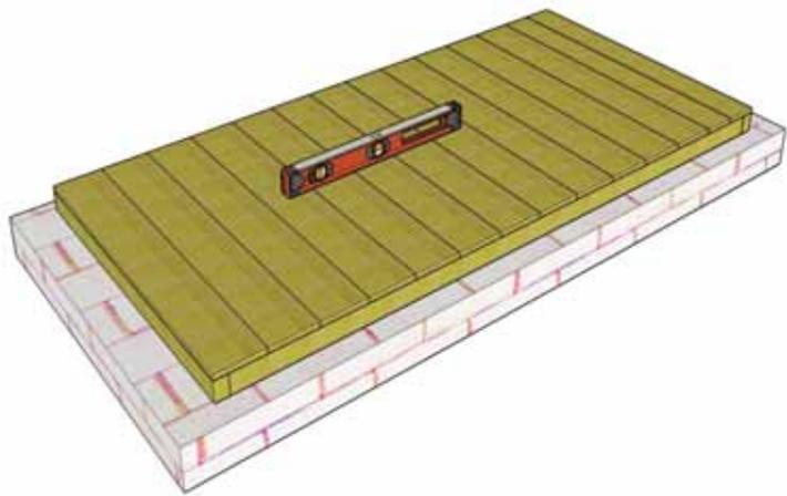
**1. Lay Chalet Floor Section (1) (35 5/8" x 74 1/4")** on a level foundation only. Patio Stones or a Concrete Slab both make excellent foundations. Use a level to confirm and shim floor joists as required.
