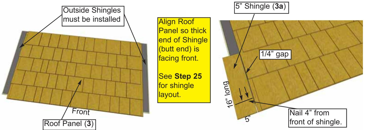
**20.** Lay **Roof Panel (3)** on flat level ground. Note, overhanging Outside Shingles have been removed to avoid shipping damage and need to be installed. Locate **(3A , 3B & 3C) Shingles**. There are 6 - 5" wide x 16" long **(3A)** Shingles, 4 - 6" wide x 16" long **(3B)** Shingles and 2 - 6" wide x 12" long **(3C)** Shingles. Position and attach **(3A)** Shingle (5" wide) on roof panel with **2 - 7/8" Shingle Nails (M)**. See above for details.
