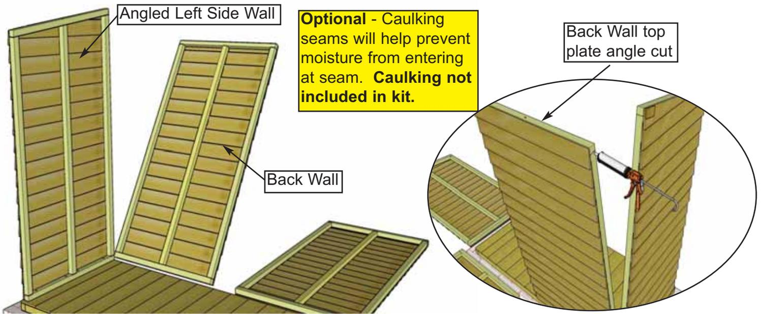
7. With your helper holding the side wall panel, position a **Back Wall Panel (2C)** in rear corner. **Important: Align Wall Siding Flush with Floor Framing.**
