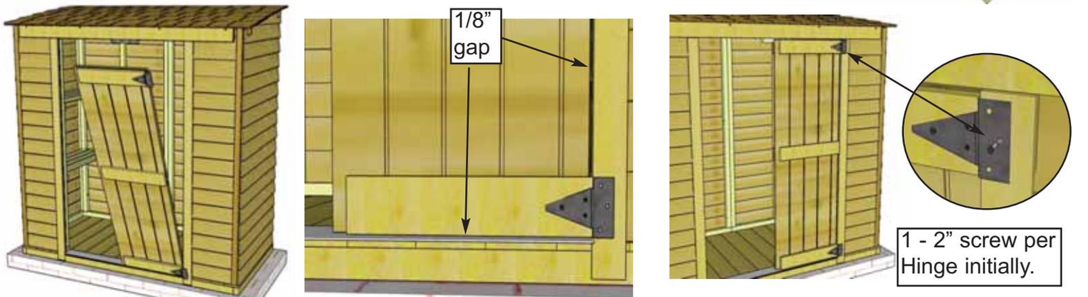
**35.** Starting with right door first, lift and position door in opening. Leave a 1/8" gap on right side and 1/8" gap on the bottom. Use a **Shim Shingle (4T)** to shim the door at bottom to help position door evenly. When door is aligned correctly, screw hinge into vertical door frame trim with **1 - 2" Black Headed Screws (H)**. Use only 1 screw initially per hinge until both door alignments are confirmed. Drill pilot holes to prevent wood from splitting.
