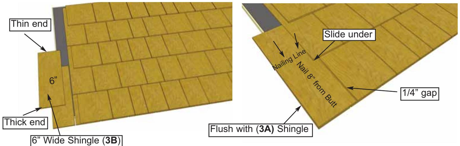
**21.** Place and attach **(3B)** Shingle (6" wide) directly on top of Shingle **(3A)**. Shingle **(3B)** will slide under 2nd row shingle. Secure with **2 - 7/8" Shingle Nails (M)** 8" from butt.
