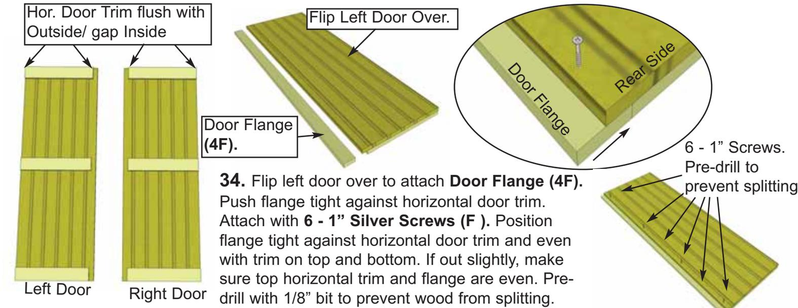
**34.** Flip left door over to attach **Door Flange (4F)**. Push flange tight against horizontal door trim. Attach with **6 - 1" Silver Screws (F)**. Position flange tight against horizontal door trim and even with trim on top and bottom. If out slightly, make sure top horizontal trim and flange are even. Pre-drill with 1/8" bit to prevent wood from splitting.
