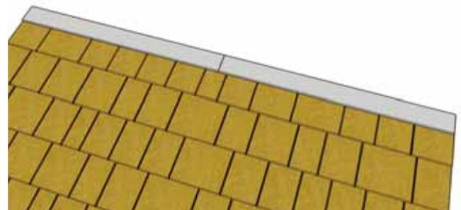
**43** Using a Step Ladder, place both **Roof Ridge Caps (4N)** (1/2" x 3 1/2" x 39") on rear row of roof shingles. Ridge Caps will overhang shingles by 1/4". Attach each piece with **4 - 1 1/2" Finishing Nails (K)**.
