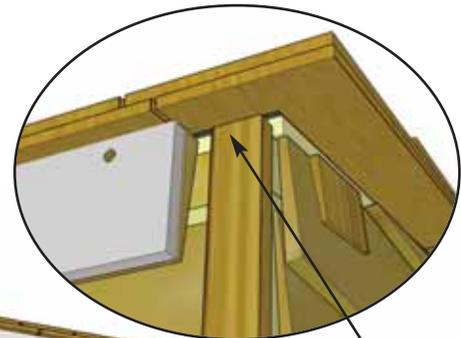
**29.** Locate **Front Horizontal Trim (4B)** (3 1/2" x 1 1/4" thick at top x 68 1/4"). Position horizontal trim tight up underneath roof panel. From side-to-side evenly space. Secure with **6 - 2 1/2" Screws (C)** into door header.
