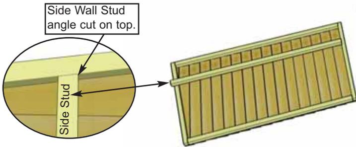
**3. Center Studs on each wall and attach with 1 - 2 1/2" Screw (C) per end. Flip walls over.**
