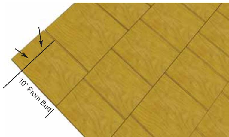
**24.** To finish end, place and attach (3C) shingle (6" wide x 12" long) in line with 5th and final row of shingles. Shingle (3C) will partially cover shingle (3B). Secure with 2 - 7/8" Shingle Nails (M) 10" from butt.
