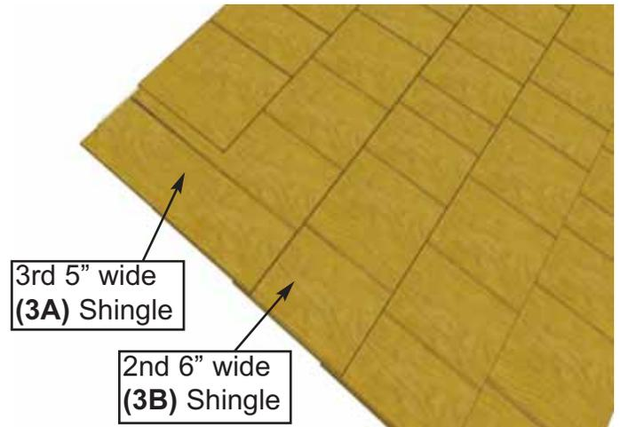
**23.** Place and attach 2nd (3B) Shingle (6" wide) in line with 3rd row of shingles. Shingle (3B) will partially cover shingle (3A). Secure with 2 - 7/8" Shingle Nails (M) 8" from Butt. Complete attachment of 3rd 5" wide (3A) shingle.
