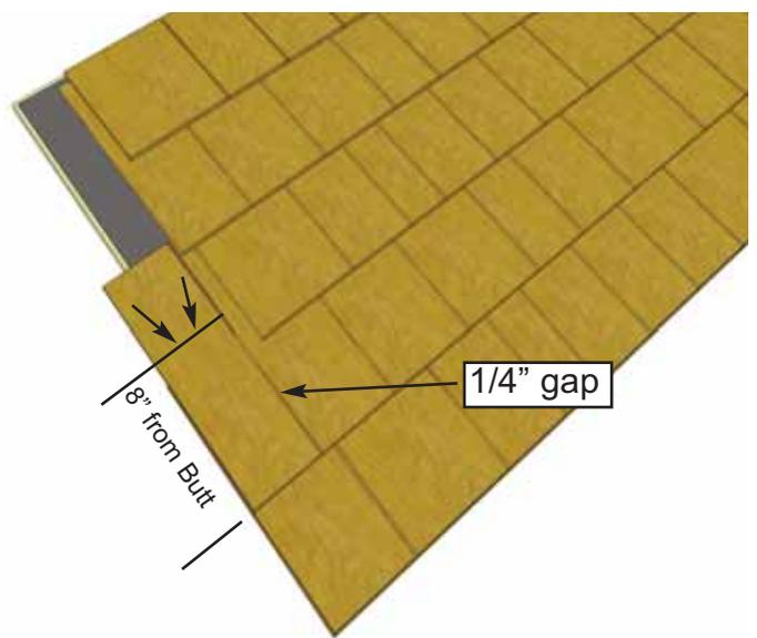
**22.** Place and attach second (3A) Shingle (5" wide) in line with 2nd row of shingles. Shingle (3A) will partially cover shingle (3B). Secure with 2 - 7/8" Shingle Nails (M) 8" from butt.
