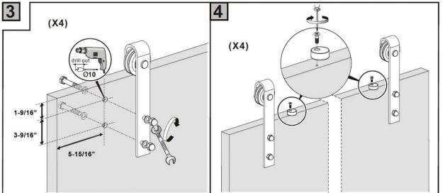
Drill out holes in the doors using a 10mm routing drill bit as pictured. The bottom of the doors should be routed at this time in order to accept the floor guide.
