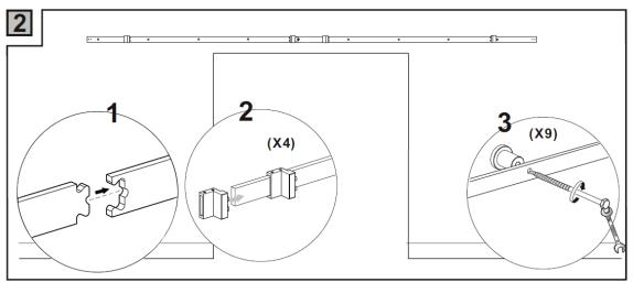
Join the two rails together. Fasten the door stops to the rail at this time, two in the center, two at each end. Attach the rail to the wall brackets using a wrench to fasten the bolts.
