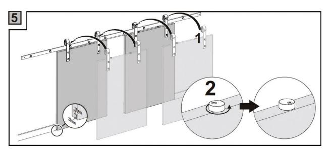
Attach the doors to the rails making sure that the anti-jump disks are engaged to avoid a serious accident.
