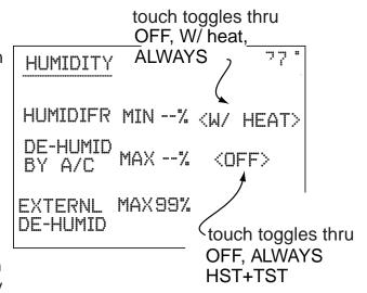
DE-HUMID BY A/C - The LS-90's humidistat can also control the Air Conditioner for de-humidifying. To set a maximum humidity level (using the air conditioner):
