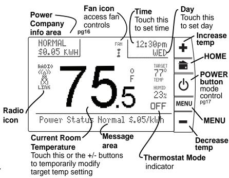
**MENU Screen** The **MENU** screen is the gateway to many functions of the LS-90. It is displayed when you press the purple MENU button on the control bar to the right side of the screen. Note page numbers for further info about each function.
