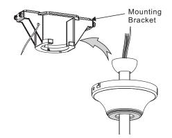
Rotate fan so that the groove on the ball engages the ridge in the mounting bracket.
