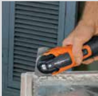
Oscillation motion eliminates risk of glass breakage.
