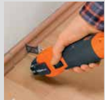
No clearance required behind the workpiece.
