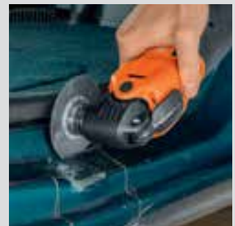
Distortion-free sawing, clean cut edges, thin cutting line – an advantage in auto body work.
