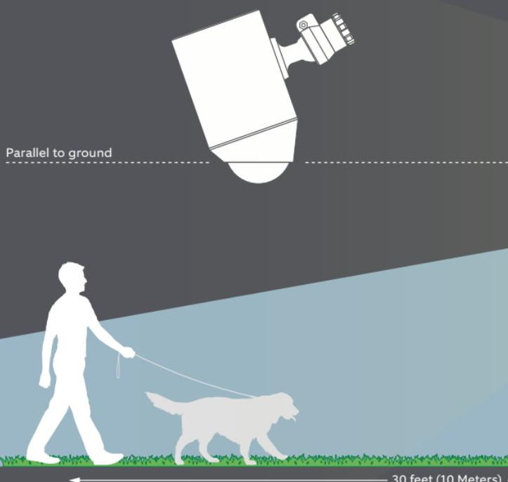
When mounted at 9 feet off the ground, with the motion detector parallel to the ground, the motion sensor is optimized to detect human-sized objects at up to 30 feet.
