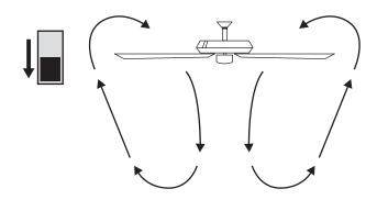
Cool weather - (Clockwise Direction) An upward air flow moves warm air off the ceiling. This allows you to set your heating unit on a cooler setting without affecting your comfort.
