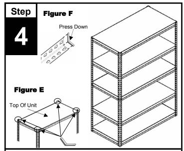
Add a woodboard shelf to the previously built level, then continue by adding the fourth and fifth level to the unit using two (2) beams and two (2) braces per level. Tap lightly to properly seat the rivets and add the final woodboard shelves to the unit. Install all four (4) end caps to the top of the unit after assembly has been completed (see figure E). Install end caps to post by pressing down on end cap at the three points illustrated above (see figure F).
