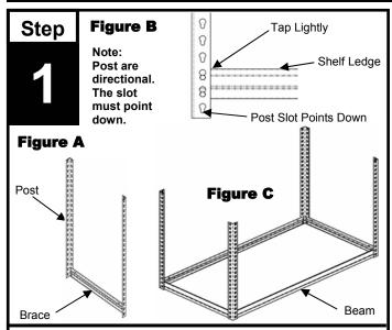
Assemble two (2) post with one (1) brace. Skipping one slot from the bottom of the post (see figure A), place the rivets into post with the slot pointing down, and with the shelf ledge of the brace facing up (see figure B). Tap lightly to seat rivets. Repeat with two (2) post and one (1) brace. Assemble the two (2) post units with two (2) beams (see figure C). Skip one hole from the bottom of post, tap lightly to seat rivets.
