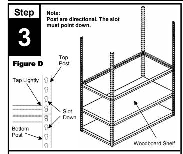
Add a woodboard shelf to the previously built level, then assemble the top post to the bottom post by using two (2) beams and two (2) braces. One (1) rivet from each beam and brace must be placed in the top hole of the bottom post, and the bottom hole of the top post (see figure D). After all beams and braces are in place, tap lightly to properly seat the rivets.
