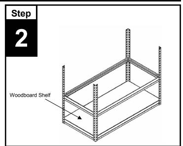
Start by adding a woodboard shelf to the level previously built, then continue working by adding the second level using two (2) beams and two (2) braces in the post slots of your desired location. Again place the rivets of the beams and braces into the post slots with the shelf ledge facing up and tap lightly to seat the rivets.
