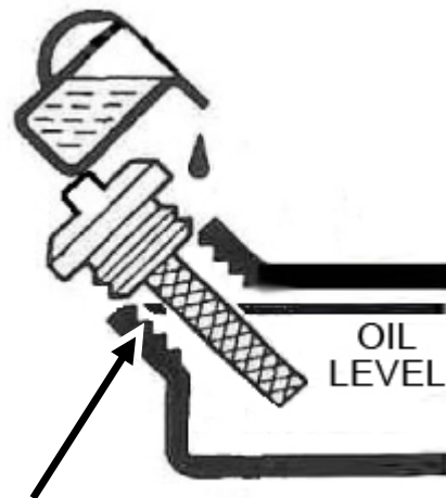
Figure 2 - Add Oil To TOP Of Threads
