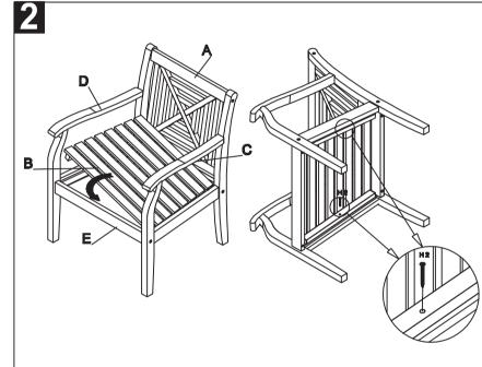
Step 1: attach right side (D) to the back (A). Then attach support L (E) and support S (F) to the right side (C) as shown on the picture by using the Allen Bolt (H1) and tighten with the Allen Key (H4). Continue with the left side (C) in the same way. Make sure to tighten all bolts (H1) before you continue with step 2.
