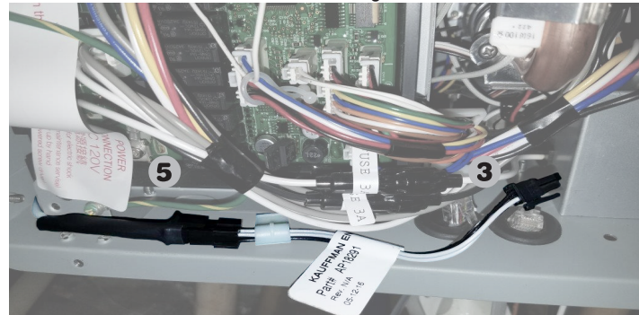
Figure 2. - Create a loop on the left side of the Gas Tankless Water Heater passing through the back of the water inlet and outlet and concluding with the tip of the sensor on the bottom-right side of the water heater. As shown in Figure 3.
