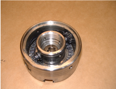
The Pinions can now come out by hand, as illustrated in the photo above.
