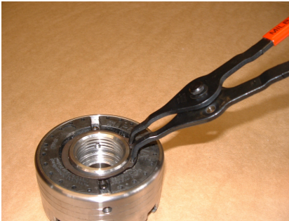
Using Circlip pliers to remove circlip
