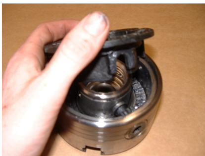
Lining up backing plate with pinions
