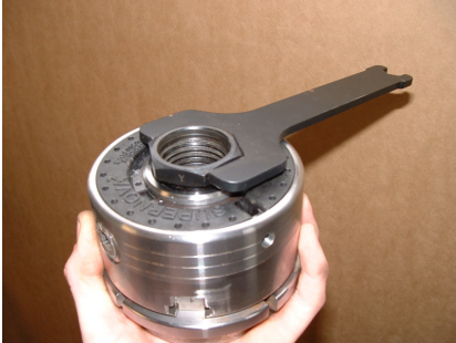
Using 1 1/2" spanner to remove insert from chuck
