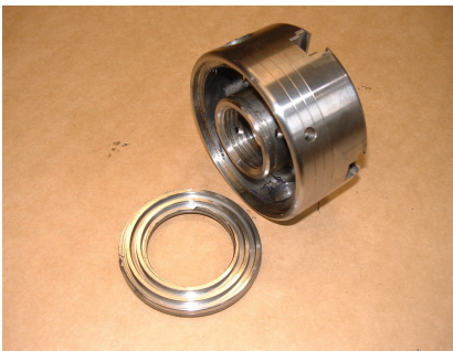
Removing scroll ring from Chuck
