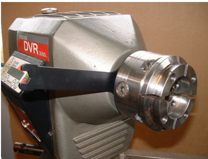
Using 1 1/2" Spanner to remove chuck from lathe
