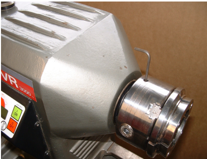
Removing grub screw to release insert
