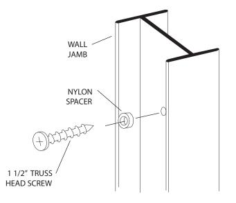
**5** This bath enclosure is equipped with safety teelock wall jambs. When installed properly, the header is permanently locked to the wall jambs and cannot be accidentally dislodged.
