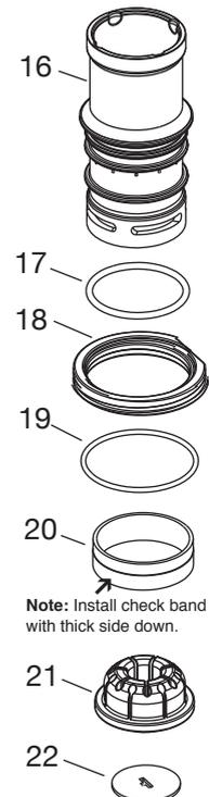
Note: Install check band with thick side down.
