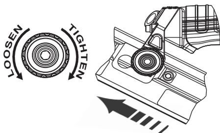
3. Slide the magazine back in the mounting bracket until the front of the magazine clears the guide pins located on the nose. Pivot or remove the magazine for inspection.
