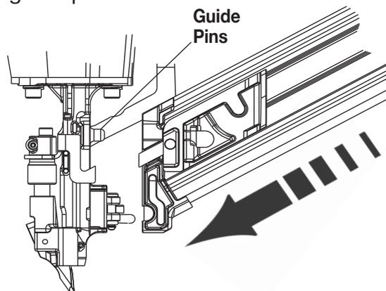
3. Slide the magazine forward inserting the nose guide pins into the magazine holes.
