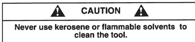
Cleaning the air-operated tools with solvents removes the thin coating of grease applied to the cylinder wall and O-rings at the factory. To replace this coating of grease, use Chemplex® grease (Paslode® Part No. 403734).
