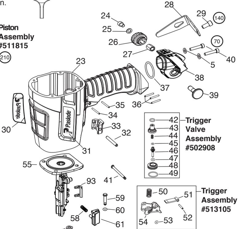
**Trigger Valve Assembly #502908**
