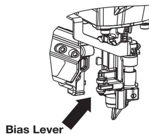
Inspect the bias lever in the nose for proper operation.
