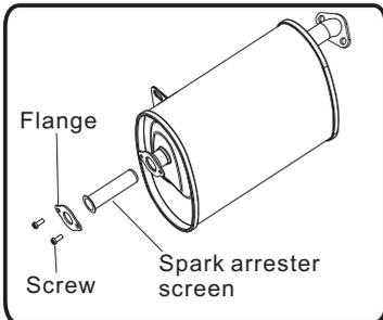
3. Carefully remove the carbon deposits from the spark arrester screen with a wire brush.
