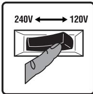
4. Plug in and turn on the desired 120 or 240 Volt AC, single phase, 60Hz electrical loads. It is better to attach the item with largest load first.
