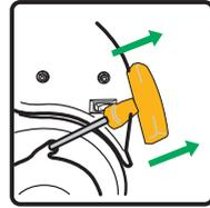
8. Do not over-choke. As soon as engine starts and warms up, move the choke lever to the "RUN" position.
