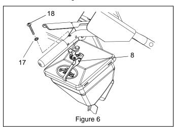
Route cable from hopper to control lever. Ensure that cable does not interfere with moving parts or controls.
