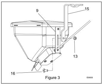
3. Position hopper assembly and top clamp (item 14) on handlebar crossbar. Secure with two 5/16 x 1-1/2 round head square neck bolts (item 12) and two 5/16 nyloc flange nuts (item 13). Ensure that hopper is level and centered on the crossbar and fully tighten hardware. Torque to 15 – 20 lbf-ft. Do not exceed 25 lbf-ft. See Figure 4.
