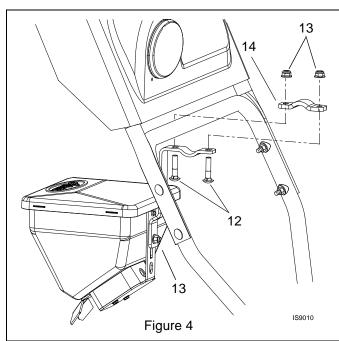
4. Position hopper at desired height and fully tighten 5/16 nyloc flange nut (item 13) installed in step 2.
