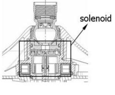
When the water flows through the solenoid,water power transfers to electricity. This electricity turns on the blue LED light.
