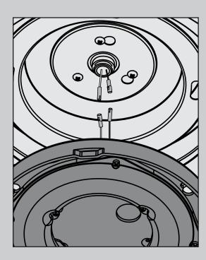
Connect the white wire from the fan to the white wire from the light kit, then connect the black wire from the fan to the black wire from the light kit.
