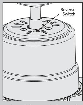
To change the direction of air flow, move the reverse switch to the opposite position.
