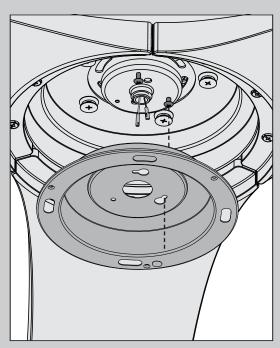
Feed the wire plugs through the center hole of the upper switch housing, then wrap keyhole slots around the screws and twist clockwise.
