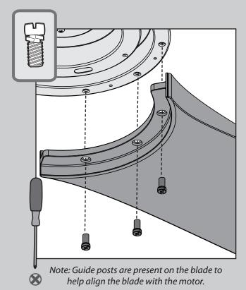
Lightly attach the blades to the motor with screws found in the ▲ hardware bag, then securely tighten after all three screws are attached.
