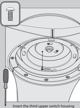
screw, found in the = hardware bag, into place and then tighten all three screws.
