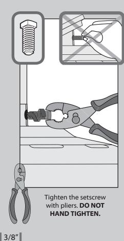
If the setscrew is not tightened securely, the fan may fall.
