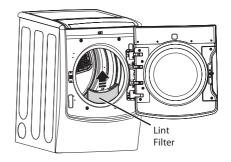
To clean, open the dryer door and pull the lint filter straight up. Then:
