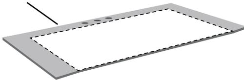
1. Ask the professional installer to make a cutout outline based on the fireclay sink; position it on the bottom of the countertop, flush to the front and centered; secure with tape.
