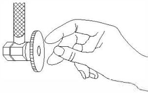
Shut off water supplies. Remove old faucet. Clean sink surface in preparation for the new faucet.
