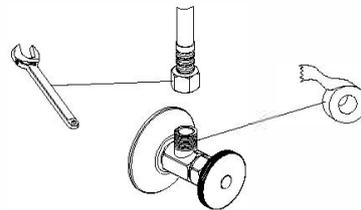
Apply pipe tape onto threads of water supplies. Use wrench when tightening the hose connection, do not overtighten.
