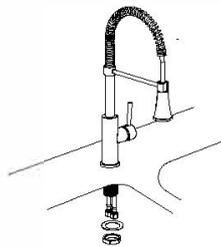
Screw the mounting stud into the body. Secure the faucet to the sink by installing steel washer and nut onto it. Tighten with wrench.
