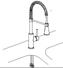
Place optional Flange on the bottom of the new faucet before positioning faucet through mounting hole.
