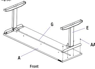
6. Attach the top rail (F) to the wood top (A), leg (B), and leg (E) using eighteen M6x15L screws (AA). Do not overtighten the screws.
