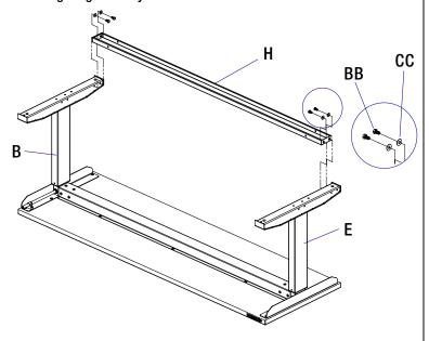
8. Square the workbench and then securely tighten all fasteners with a 10 mm and 13 mm wrench.
