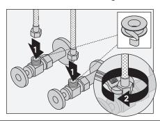
**Optional:** Adjust limit stop washer to limit handle turn to the hot position if desirable.
