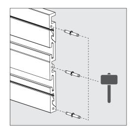
If your having trouble getting dowels into dowel holes by hand you can tap dowels lightly with a hammer or mallet.
