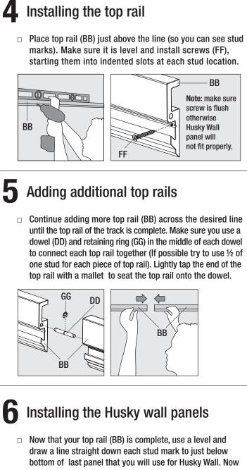
take each Husky Wall panel (EE) and slide into top rail (BB), which will cover screws from previous steps.
