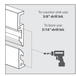
If there is a gap between two top rails end to end or bottom rails end to end because of the dowel / e-clip you can counter sink the hole 1/8" with a 3/8" drill bit.
