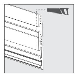
If side rails don't fit because the panel, top rail, or bottom rail are too long use a saw to cut off extra length.
