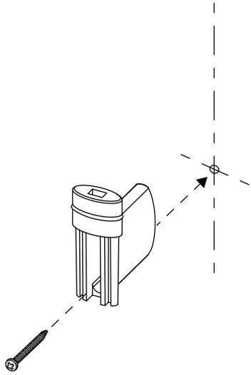
Locate the bottom bracket in the desired position and attach with one screw.
