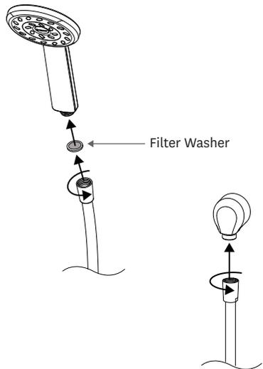
For handset only installations remove existing hose. Insert the filter washer into the new hose before screwing to the handset.
