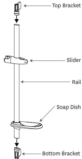
Attach the slider and the soap dish to the rail in the desired orientation. Fit the rail to the bottom bracket. Fit the top bracket to the rail.
