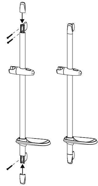
Insert the remaining screws. Fit the end caps.
