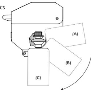
**Valve will feel loose and will rotate easily. Even though the valve feels loose, it is designed that way and will not leak. The valve was designed to be loose fitting in order to allow safe, easy installation and removal of the propane canister and so it easily swings without resistance to fit all applications**
