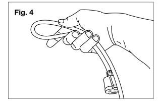
Insert the loop through the hole in the back of the upper handle, securing the loop around the hook.
