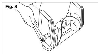
2. Remove the old rotor from the housing.
