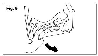
**3.** Install the new rotor in the housing by inserting the end of the rotor onto the fitted end in the housing and rotating the rotor until it snaps into position.
