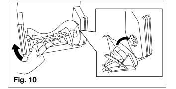
4. Tighten the bolt on the side of the housing.
