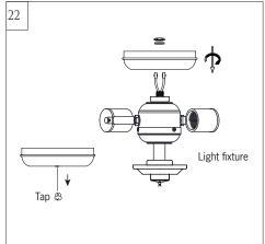
Remove the tap from bottom of the switch housing cap.
