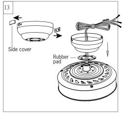
Remove side covers from canopy exposing 4 holes. 2 closed holes and 2 open "L" shape holes.
