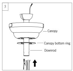
Place downrod over canopy and canopy bottom ring. Thread lead wires and safety cable from motor assembly through downrod.
