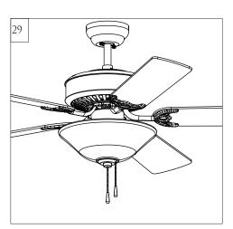
Install fan and light kit pull chains to preassembled pull chains on fan. Pull chains provided.
