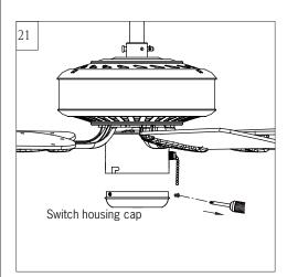
Remove switch housing cap by removing the set screws. Keep screws.
