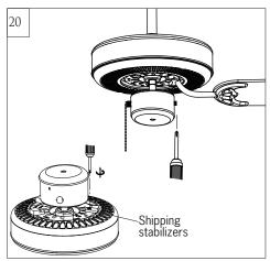
Remove shipping stabilizers from motor assembly.
