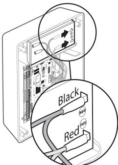
Position battery in control box as shown.
