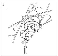
Attach the light fixture onto the light pan , aligning its keyhole slots with the preassembled set screws on the light pan and twist clockwise till lock. Reinstall the screw removed in step 15. Tighten all screws securely.
