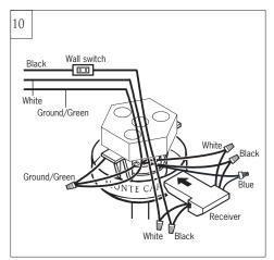
Make wiring connections using wire connectors provided as indicated above. White from fan to White from remote marked N. Black from fan to Black from remote marked L. Blue from fan to Blue from remote marked FOR LIGHT. White from house to White from remote marked AC N. Black from house to Black from remote marked AC L. Connect all green grounded wires to Grounded wire from House. Make sure that no filaments are outside of the wire connectors. Insert the remote receiver into mounting bracket.
