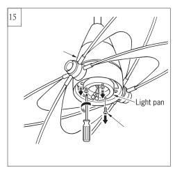
Loosen 2 and remove 1 preassembled set screws from light pan. Save screw for later use.
