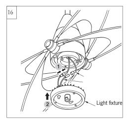
Connect white wire from fan to white wire from light fixture. Then connect black wire from fan to black wire from light fixture.
