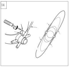
Align the screws holes in blade frame and the holes in the coupler and then fix the blades in the couplers with set screws provided.
