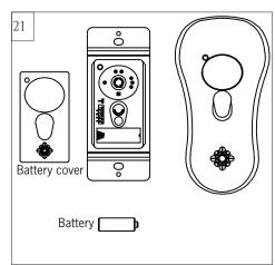
Remove battery cover. Install 12V battery into wall remote. Duracell MN21 / Evereday A23 / GP 23A all 12V. Attach cover of remote by placing over buttons and snap the battery cover in place.
