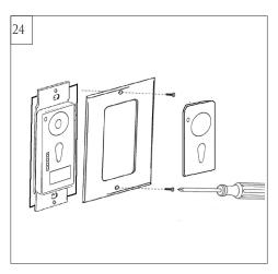
Attach front cover to wall control unit with screws provided. Snap battery cover in place
