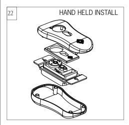
Place battery cover over battery compartment and buttons. Place remote over 2 pins on front cover. Attach cover of remote by placing over 4 pins and snapping into place.
