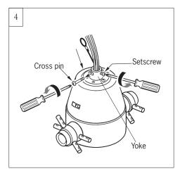
Remove cross pin from yoke at top of motor assembly. Keep it for later use. Partially loosen downrod set screws from yoke at top of motor assembly.
