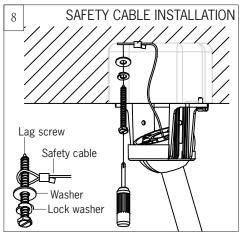
For Canadian installation and for USA fan and light kit combinations over 35 lbs, in both flush and downrod modes the safety cable must be installed into the house structure beams using 1.5" lag screws, washers and lock washers provided. Make sure that when the safety cable is fully extended the lead wires are longer than the cable and no stress is placed on the lead wires.
