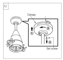
Lift canopy up, aligning its keyhole slot with the preassembled screw on mounting bracket and twist counterclockwise to lock in place. Reinstall the screw removed in step 11 and tighten all screws securely.
