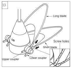
Insert the short blade into the lower couplers and then insert the long blade into upper couplers on the hubs. Repeat this process for the remaining blades assemblies on the other side of the hubs. **Note**: Make sure the screw holes in blade frames are installed upward.
