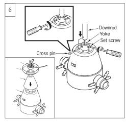
Slip downrod into motor housing yoke, aligning holes and Reinstall the cross pin. Insert cross pin through yoke and downrod and then fasten it with screwdriver. Pull the downrod up tight against the cross pin, and then evenly tighten the downrod set screws on motor housing yoke.
