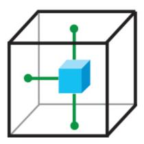
DEWALT offers spot lasers in both 3-spot and 5-spot. A 3-spot provides plumb and forward-facing dots whereas the 5-spot adds a right and left dot for transfer of points from wall to wall. A suggested SKU is our Green Beam 3 Spot Laser (DW083CG) with a high-visibility green beam. This laser includes a single lever power switch that locks the pendulum in the off position, as well as a built-in magnetic pivoting bracket to easily mount the laser onto metal surfaces.
