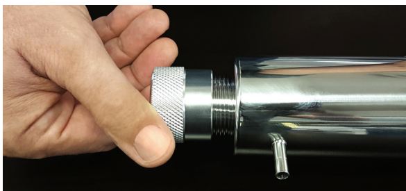
5. Screw the Metal Cap onto the UV Housing. Use a wrench to finish tightening, do not over-tighten. DO NOT TOUCH UV BULB DIRECTLY, USE THE WHITE CERAMIC PORTION TO MOVE THE BULB!
