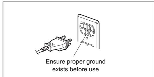
For a permanently connected appliance: This appliance must be connected to a grounded, metallic, permanent wiring system, or an equipment grounding conductor should be run with the circuit conductors and connected to the equipment grounding terminal or lead on the appliance.
