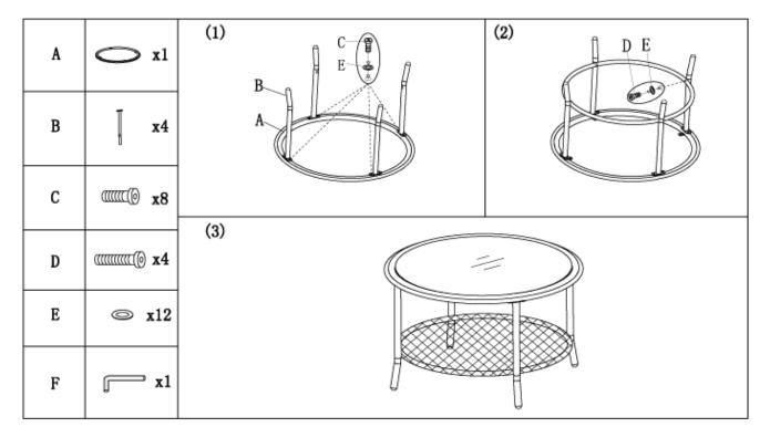
Note:do not tighten bolts until all parts are connected
