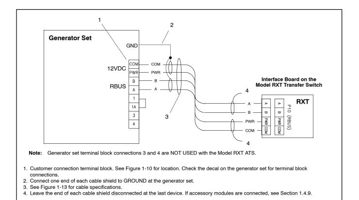
Figure 1-11 Model RXT Transfer Switch Communication Connection to Generator Set Terminal Block
