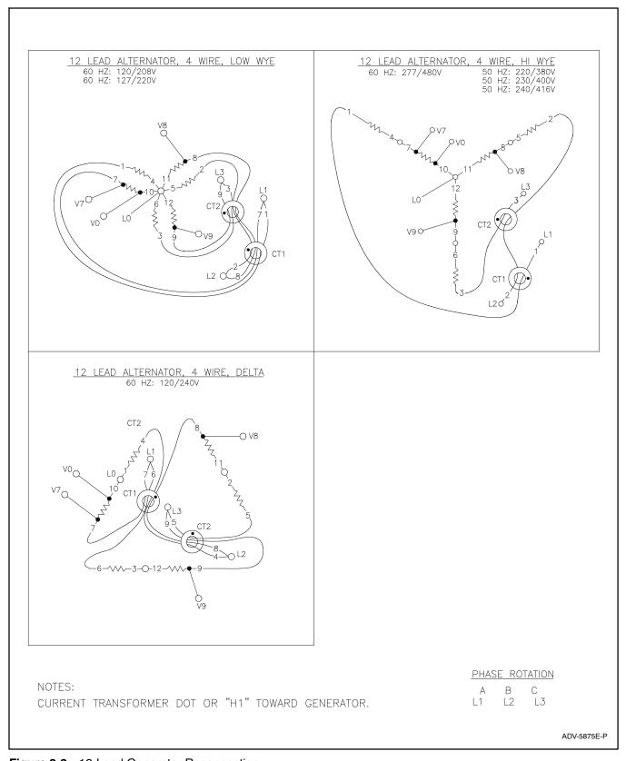
Figure 3-2 12-Lead Generator Reconnection
