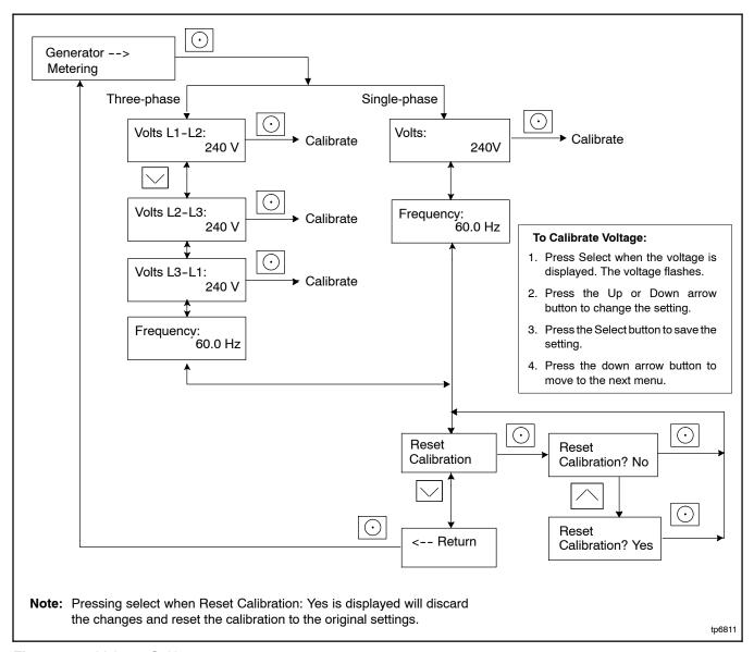
Figure 3-6 Voltage Calibration
