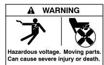
Operate the generator set only when all guards and electrical enclosures are in place.
