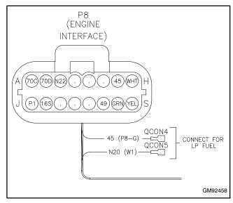
Figure 1-21 Fuel Type Connections
