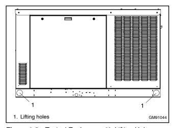
Figure 1-2 Typical Enclosure with Lifting Holes
