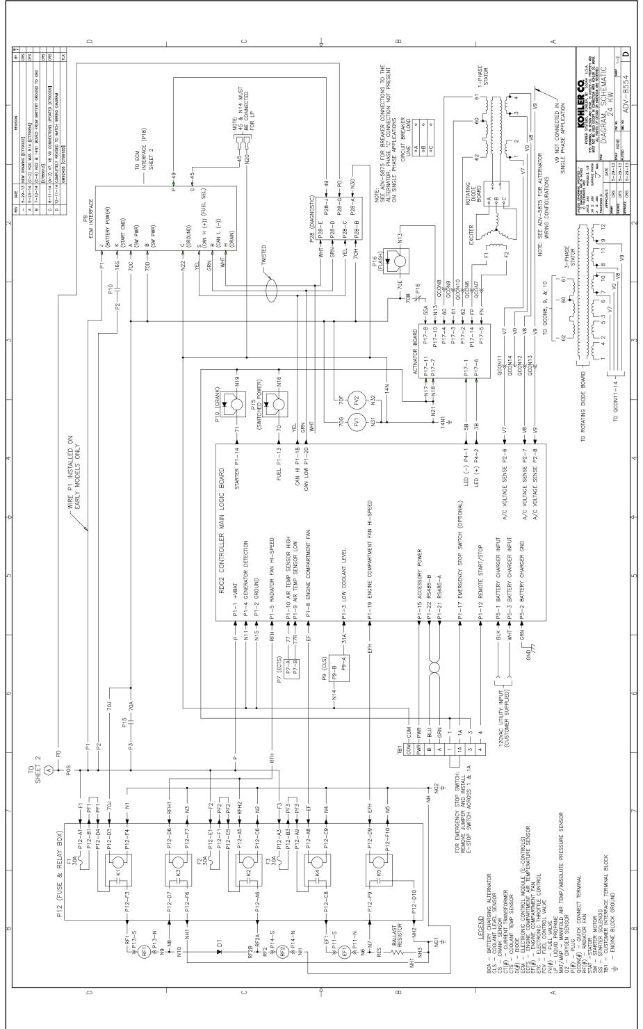
Figure 4-2 Schematic Diagram, 24RCL Generator Set, ADV-8554, Sheet 1 of 2
