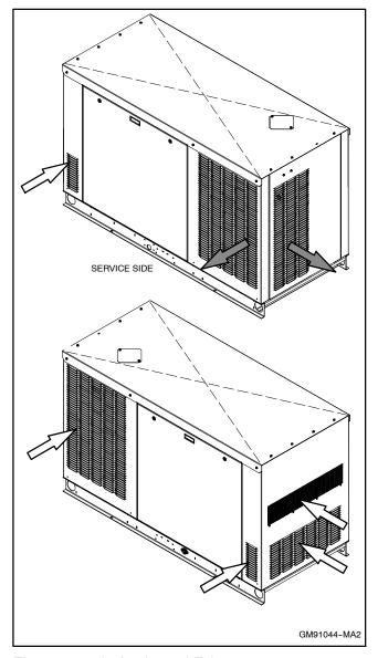
Figure 1-5 Air Intake and Exhaust
