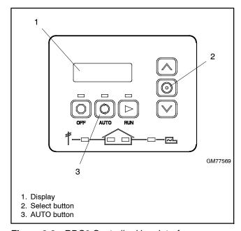
Figure 3-3 RDC2 Controller User Interface
