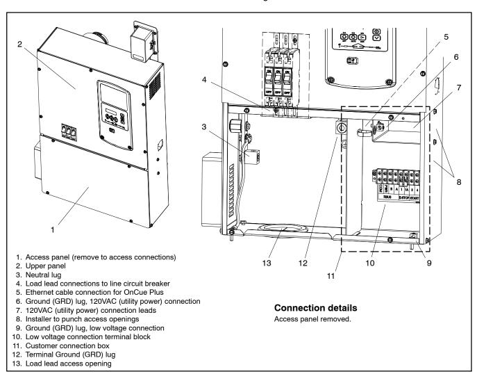
Figure 1-10 Generator Set Connections
