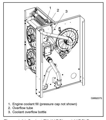
Figure 1-24 Coolant Fill (30RCL and 38RCLB shown)
