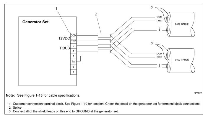
Figure 1-16 Multiple Connections to the Generator Set
