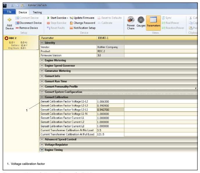
Figure 3-8 Voltage Calibration Factor in SiteTech™
