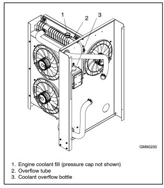
Figure 1-23 Coolant Fill (24RCL shown)
