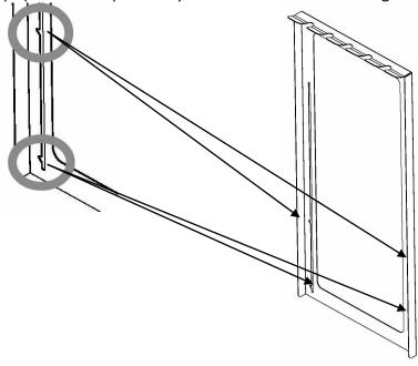
23. To retract the tool holder, remove all tools, and loosen all 4 plastic head screws. Now lift the tool holder slightly to take it off the "hooks" and gently allow it to slide down in to the storage position.
