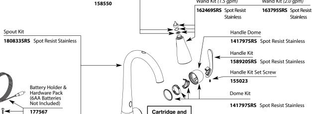
Cartridge and cartridge nut are not serviceable items.
