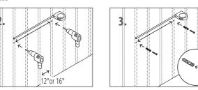
1. Measure the distance between the screw holes from the 2. Locate the studs on the wall. They are normally placed 12" to 16" apart from each other. Drill two holes on the studs as 3. Insert the plastic plugs into the drilled holes and then insert screws into the plastic plugs. Tie up the screws till they 4. Hang the mirror on to the screws.
