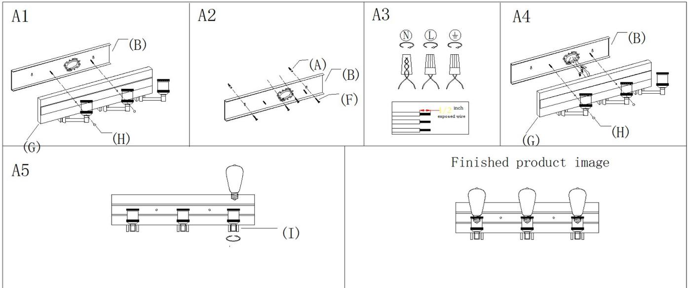
Step A1: Unscrew the knob nut(H) from back plate(G) then gently remove mounting plate (B)
