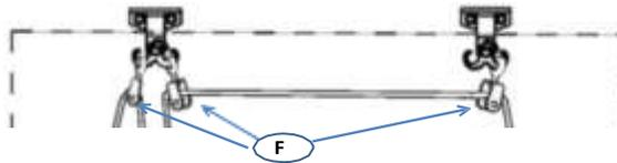
3. Assemble the Head Rod bar using the internal connector.
