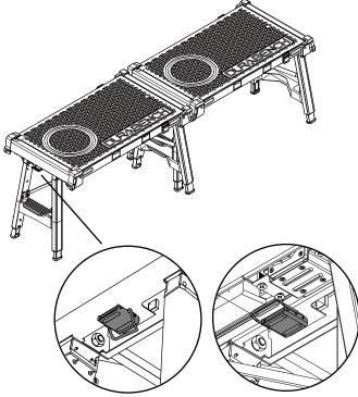
Make sure the lock is locked on.
