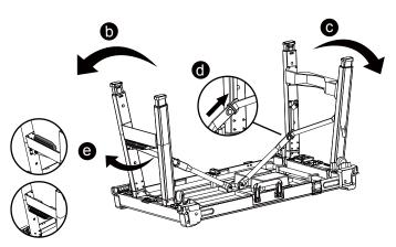
NOTE: You must open the narrower set of legs first, then the wider set of legs. Otherwise the legs can not open.
