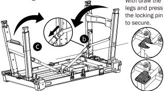
NOTE: You must close the wider set of legs first, then the narrower set of legs. Otherwise the legs will not close properly.
