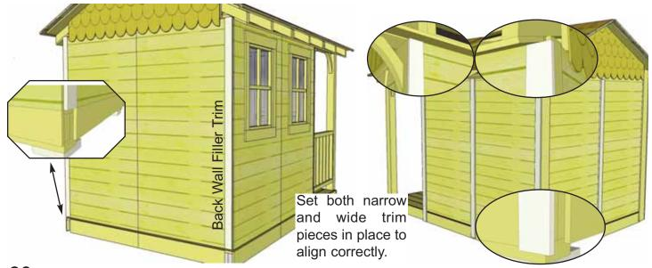
**60.** Attach two 1/2" x 2 1/2" x 60" **Back Wall Filler Trims** to back wall corners. Hammer with 6 - 1 1/2" finishing nails. Flush trim with skirting and siding.
