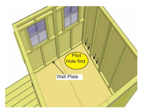
**17.** When all walls are attached together, check alignment with the floor. Bottom Wall Plates should sit flush with outside of Floor Framing. When positioned correctly, fasten Bottom Wall Plates to floor using 4 - 2 1/2" screws per Wall Panel.
