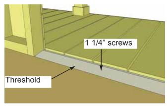
**68.** Also included is an optional **Doorway Threshold** piece that is 23" long and angle cut. Attach where Plywood Floor and Decking meet under the door with 3 - 1 1/4" screws.
