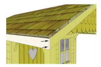
**64.** Attach **Side Facia** to Roof Rafter Ends. There are two Side Facia pieces per side. Secure with 8 - 1 1/2" finishing Nails per piece.
