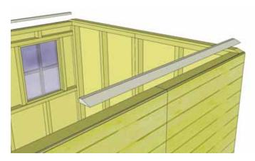
When in correct position, screw down plate with 4 - 2" screws per piece.
