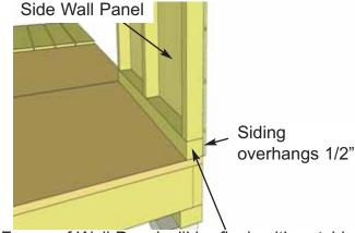
Frame of Wall Panel will be flush with outside of Floor Frame when properly aligned.
