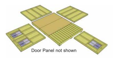
9. Lay out all the Wall Panels and become familiar with their location. On Standard Kits, there are 3 Window Wall Panels and 4 Solid Wall Panels. All wall panels are 35" wide x 60" high and can be placed in any location, except for the Door Panel (not shown to the left). The Door Panel must be positioned to the left front. NOTE: You must attach Wall Plates to the bottom of all Solid Wall Panels. Window Inserts for Window Walls will need to be positioned and attached as Per Step 11.
