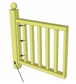
Use Rail Support Block (3 1/2" high) from bottom of post to align rail. Attach rail to post with 3 - 2" screws.
