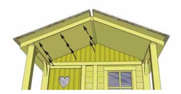
**53**. Position Porch Veneer with best face exposed, flush with front Rafter and Ridge Board. When correctly in place, nail veneer to rafters with 12 finishing nails. Complete both sides.
