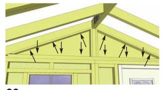
**39.** Secure Rafters to Middle Gable Wall framing and Top Wall Plates with 12 - 2" screws.
