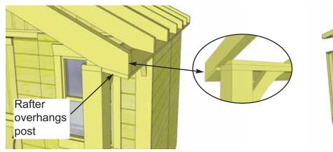
**35.** Rafter will overhang Porch Post when correctly positioned on walls.
