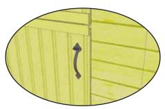
**19.** Attach **Door Handle** and **Interior Silver Barrel Bolt** Hardware. Use 3/4" Black Headed Screws to secure the Door Handle. **Important:** Drill shallow Pilot Holes to prevent wood from splitting. Align male and female Barrel Bolt to Door Framing. Attach with 3/4" Black Headed Screws.
