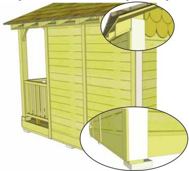
**63**. Attach **Facia/Roof Nailing Strips** to the underside edge of the plywood roof. Center and attach with 3 - 1 1/4" screws. Complete all four sides.
