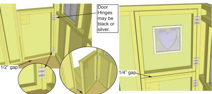
**18.** Attach 2 Hinges (top and bottom) to Bottom Door framing with 3/4" Black Headed Screws. Position the Door into door opening. Leave a 1/2" gap between floor and bottom of door framing. Use Spare Shingle to help shim door into proper position. Initially, secure Door to Door Jamb with one screw per hinge. Check door alignment by moving door back and forth. When satisfied with position, completely secure Door to Door Jamb. Follow same procedure for Top Door leaving 1/4" gap between doors.
