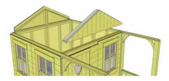
**27.** Position the **Middle Gable Wall** on top of Front Top Plate. When in correct position, attach with 2 - 2" screws as per **Step 26**. Complete installation in **Step 39**.
