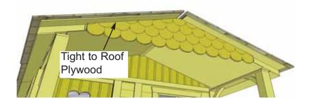
**55.** With Decorative Gable correctly positioned, fasten to rafters with 4 - 2" screws (2 per side). Drill 1/8" pilot holes first to avoid splitting the decorative shingles.
