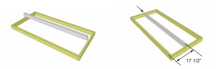
1. Floor Joist Frames require one interior Floor Joist attachment each. Center Floor Joist (17 1/2" from outside of Frame to center of Floor Joist) and attach with 2 - 2 1/2" screws per end. You can find the Square Drive Bit for the screws in with the Hardware Kit Bag.
