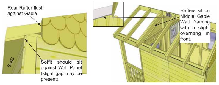
**34.** Position Rear Rafters flush against Rear Gable. On the Middle Gable, Rafter will slightly overhang siding of Middle Gable Wall.
