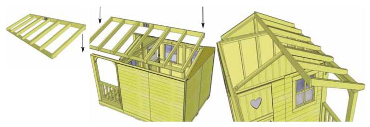
**32.** Flip Rafter Section over so Soffit is down. Carefully lift completed Rafter Section up and place on middle and rear Gable Framing.
