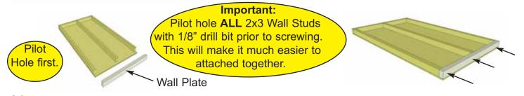
**10.** Starting with **Solid Wall Panels**, carefully lay panel face down. Position and attach **Wall Plate** to bottom of wall studs of each Panel with 3 - 2 1/2" screws. Position so plates are flush with framing.
