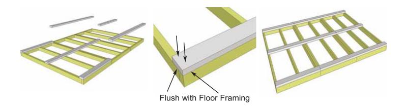
**4.** Attach **Floor Runners** to completed Floor Joist Frames. There are two Floor Runners per 105" side and three completed Floor Runners in total. Use 6 - 2 1/2" screws per Runner to secure.
