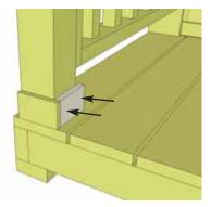
**58.** Attach **Post Base Trims** to bottom of Porch Posts. Attach with 1 1/4" finishing nails. Center a **Rail Support Block** (1 1/2" x 3 1/2" x 3 1/2") under each Handrail Section and secure from top down with 2 - 2 1/2" screws. Complete each Handrail Section.
