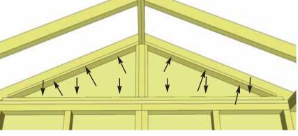
**38.** With both Rafter Ridge Boards connected, secure Gable Framing to both Outside Rafters and Top Wall Plates with 12 - 2" screws.
