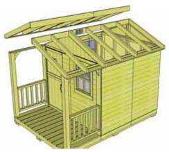
**36.** Place second completed Rafter Section on Gable Walls and position as per **Steps 32 - 34.**
