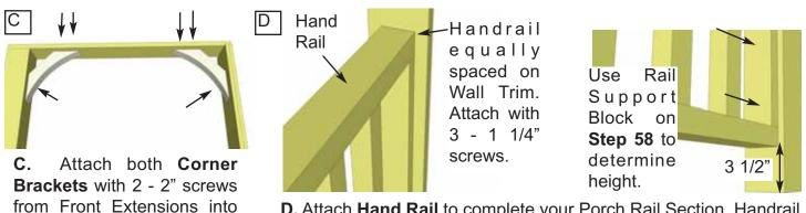
**D.** Attach **Hand Rail** to complete your Porch Rail Section. Handrail should start 3 1/2" from bottom of Post and be centered on Trim and Post. Attach with 3 - 1 1/4" screws on Trim side, and 3 - 2" screws on Post side.
