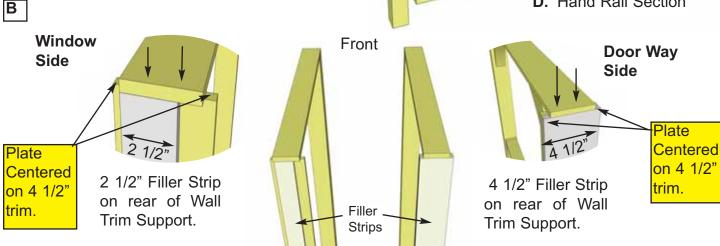
**B.** Attach 1x4 1/2" **Wall Trim/ Supports** to Front Extension using 2 - 2" screws. Make sure Front Extension is Flush to back of wall trim and centered 1/2" on each side. **Note:** there are 2 different wall supports for left & right. See diagram for proper orientation.
