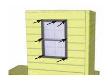
**11a.** Position Window Trim around window doing a dry run first and attach with 4 - 1 1/2" finishing nails per piece. The window kit trim pack = 1x 24 1/16" = top / 3 x 23" = sides and bottom. Window trim has a small dado on reverse face. Outside flange of window will roughly sit in the dado to give a better fit.
