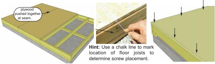
7. When Plywood Floor is correctly positioned, attach with 1 1/4" screws. Use screws every 16".
