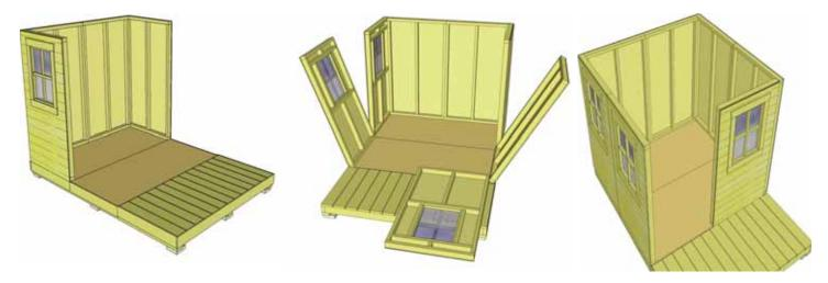
**14.** Continue to attach walls, working your way around the playhouse. Once again, screw walls together using 2 1/2" screws at the top, middle and bottom of Wall Studs.
