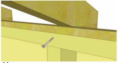
**41.** Secure Rafters to Top Wall Framing with one 3" screw per rafter. Screw through Wall Frame at an angle. Prior to attaching, make sure walls are properly aligned. Have two helpers push the side walls at the top from the outside of shed until inside to inside measurement between side plates is 70".
