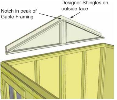
**26.** Position the **Rear Gable Wall** on top of the Rear Top Plate. The Rear Gable can be distinguished from the other two gables because it has Designer Shingles protruding below frame. Temporarily attach to walls and top plate with 2 - 2" screws. Gables may need slight adjustment in **Step 38.** Complete attachment when correctly aligned in **Step 38** with an additional 6 - 2" screws.
