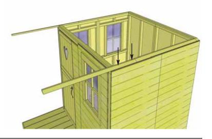
**24.** Complete the **2 Porch Rail Sections**, following steps **A** through **D**. **Note:** Sections differ - see step B for orientation.
