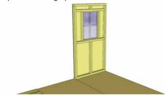
**13.** The Side Wall Panels will sit flush at the end of the Plywood Floor with the front and rear panels sandwiched between them. **NOTE:** Siding will overhang the floor by approx. 1/2". Position Rear Solid Wall on floor in corner and attach vertical wall studs together with 3 - 2 1/2" screws.
