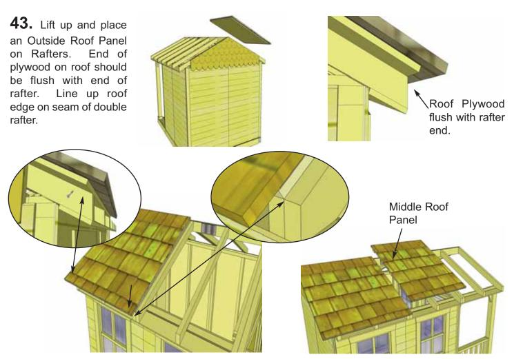
**44.** Place Outside Roof Panel so it sits flush on 3rd rafter from the outside (doubled up rafter). Plywood on roof should be flush with end of rafter at bottom. From the outside, screw down through bottom row of shingles into rafter with 1 - 2 1/2" screw. Angle a 2 1/2" screw from outside rafter into roof plywood. Locate **Middle Roof Panel** and position on Rafters.
