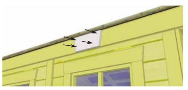
**67.** Attach **Pentagon Facia Plate** to Rear and Front Facia with 4 - 1 1/4" finishing nails. Facia Plate will cover any gaps existing where Facia's come together at peak. Attach **Facia Detail Plates** (2) where Side Trims meet. Use 4 - 1 1/2" finishing nails to secure.
