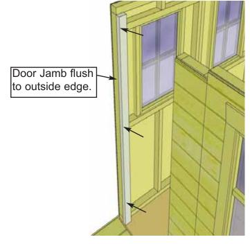
**16.** Attach the **Left Side Door Jamb** to Left Side Wall Stud. Make sure Door Jamb is flush with floor and flush with existing wall stud. Use 3 - 2 1/2" screws to secure. Next, attach the **Door Header** to Door Jamb and Top Plate of Narrow Wall. Use 3 - 2 1/2" screws to secure. **IMPORTANT:** Check door opening measurement at top and bottom. It should be 23 1/2".
