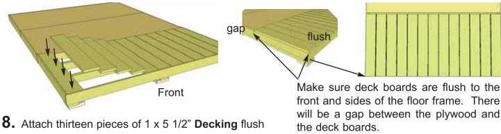
**To a stack thirteen pieces of 1 x 5 1/2" Decking flush** to front using 4 - 2" screws per piece. With Decking, attach both outside pieces first and equally space all others on the floor before attaching.
