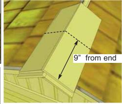
Important - Butt (thick) end of Ridge Cap will be facing towards the outside of shed.
