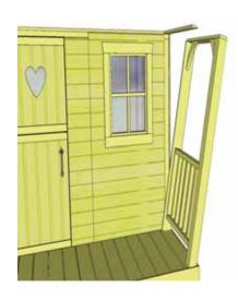
**25.** When both Porch Rail Sections are complete, lift into place on Playhouse Deck and beneath the Side Top Plate. (Window Side section will have Narrow Filler Trim). Position so Post is flush with Decking on the side and recessed 1/2" in the front. Attach wall support to playhouse wall with 3 - 2 1/2" screws. Try to conceal screws if possible.
