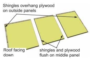
**42.** Identify all **Roof Panels**. There are four **Outside** and two **Middle Roof Panels**. Outside Panels will have shingles overhanging the plywood on one end.
