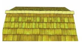
**66.** Place 3rd Ridge Cap 8" back from 2nd (enough to cover shingle nails). Attach 3rd Ridge Cap down as per **Step 65.** Continue to position and attach Ridge Caps until half the roof is complete. From opposite side, position and attach Ridge Caps as described above. Score/cut 1 Ridge Cap to 12" or to fit in the center of roof. Attach center cap with 4 - 1 1/4" Shingle Nails.
