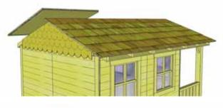
**47.** Position and attach all remaining Roof Panels as per **Steps 42-46**.
