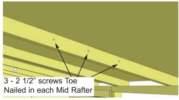
**52.** To further secure roof panels, from the inside, drill pilot holes in each Mid Rafter (3 per Rafter) on an angle. Using 3 - 2 1/2" screws, secure rafters to roof plywood. **Note:** from outside, have a helper push roof panel down so plywood sits flush against rafter when securing. In Porch area, angle screw both the mid and outside rafters.
