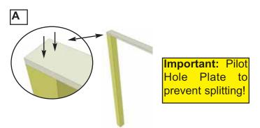
**A.** Attach 1x4 **Top Plate Front Extension (34 1/2"L)** to 4x4 Porch Post with 2 - 2" screws. Make sure support is flush with post.
