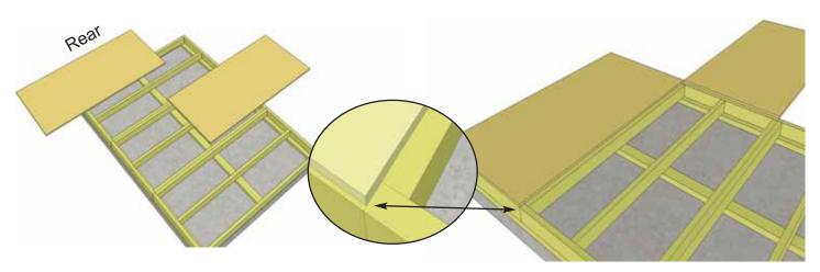
**6.** Position **Plywood Floor** pieces (2) on top of completed Floor Joists. Plywood is cut slightly smaller than floor framing. Keep plywood seam tight.
