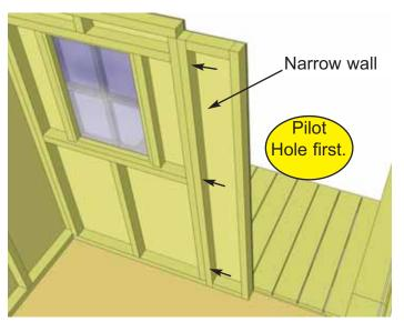
**15.** To attach the Door, first position the **10" wide Narrow Wall** next to the Window Wall and screw into adjoining wall stud with 3 - 2 1/2" screws.
