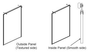
B. Use two more #8-32 x 3/8" HWH Screws (#17) to attach two Rollers (#10) to the top of the Inside Door Panel (#6) of the frame on the back surface of the "fin", with the metal parts (the Nut side) against the frame and the plastic Roller (#10) facing into the shower (the same side as the smooth side of the glass).
