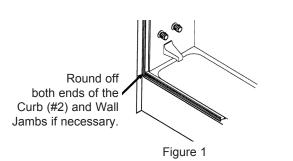
B. Locate the Curb (#2). Cut the Curb (#2) 1-1/16" shorter than this measurement. If your shower has curved corners, use a File to round off and shape the ends of the Curb (#2) to fit the rounded corners (See Figure 1). **Do not cut the Header (#1) at this time.**
