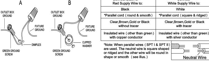
Twist plastic wire connector (A)until wires are tightly joined together, wrap each connector with approved electrical tape and carefully tuck all wires into the outlet box .
