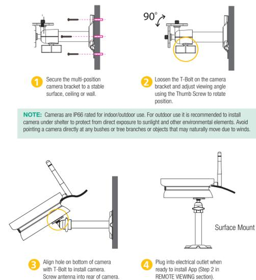
**NOTE:** Cameras are IP66 rated for indoor/outdoor use. For outdoor use it is recommended to install camera under shelter to protect from direct exposure to sunlight and other environmental elements. Avoid pointing a camera directly at any bushes or tree branches or objects that may naturally move due to winds.
